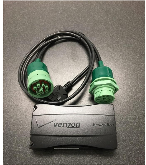
1 the unit that is installed in the truck/not much bigger than a cell phone
